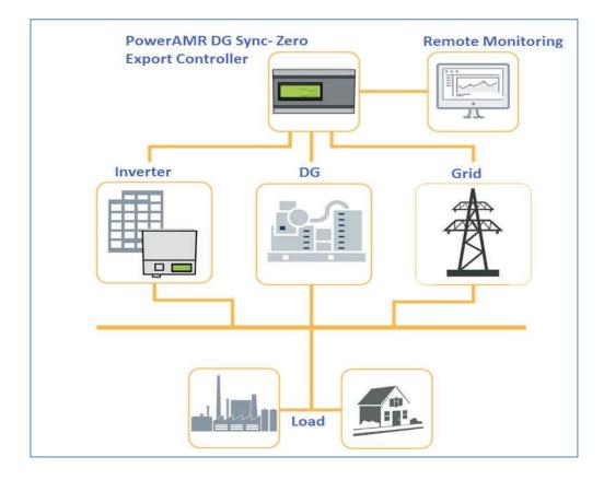
This solution has common facility for DG –Solar syncing as well as Zero export. When the grid is available, it will work as Zero export solution and when DG is available for Reference voltage, it will work as DG-Solar sync solution.
