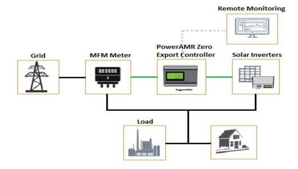
This solution is working when grid is available but there is no net metering at site. The zero export solution will help user to use solar as per demanded load. This solution will throttle the power of solar inverters as per building load and there will be No Export to grid.
